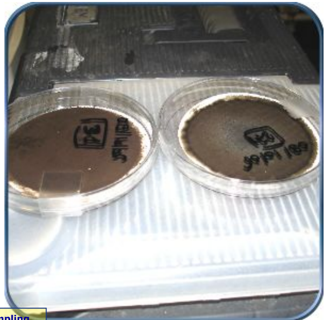
Sulfur sampling and particulate sampling filter
